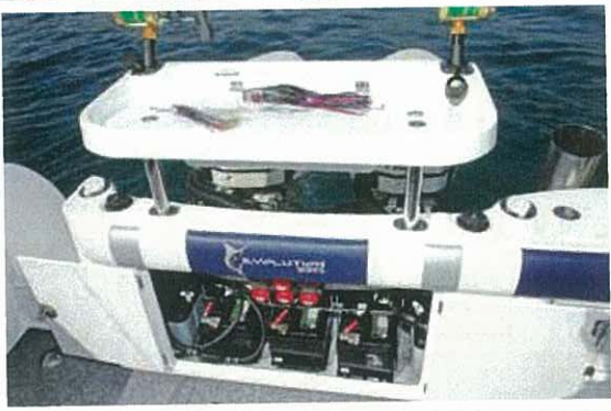
Left: A well laid out helm puts it all at your fingertips. Above: Well crafted rod storage and gaff racks keep your tackle well organised. Below: Twin doors reveal the battery compartment and isolator switches.
