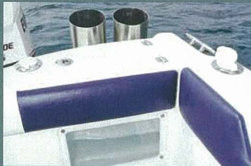
Above: Plumbed tuna tubes and a viewing panel on the livebait tank are nice additions. Below: The step-up walkway to the bow.
